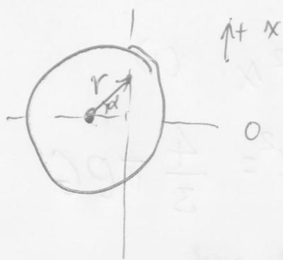
$\alpha$  is angle between middle of tunnel and vertical direction.
